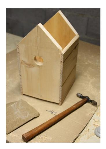
The roof needs to be finished with roofing felt or similar to keep out the rain. It's best to provide overhangs to all sides to throw off rainwater and provide shading from direct sun.
